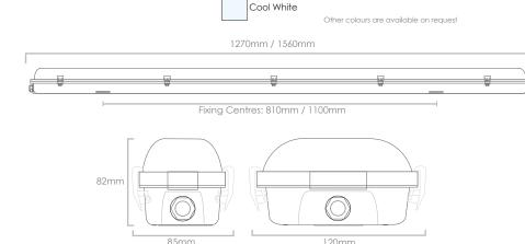
Industrial Lighting / Linear LED IP65 Non-corrosive Fitting / 4ft Twin / 5ft Single / 5ft Twin
